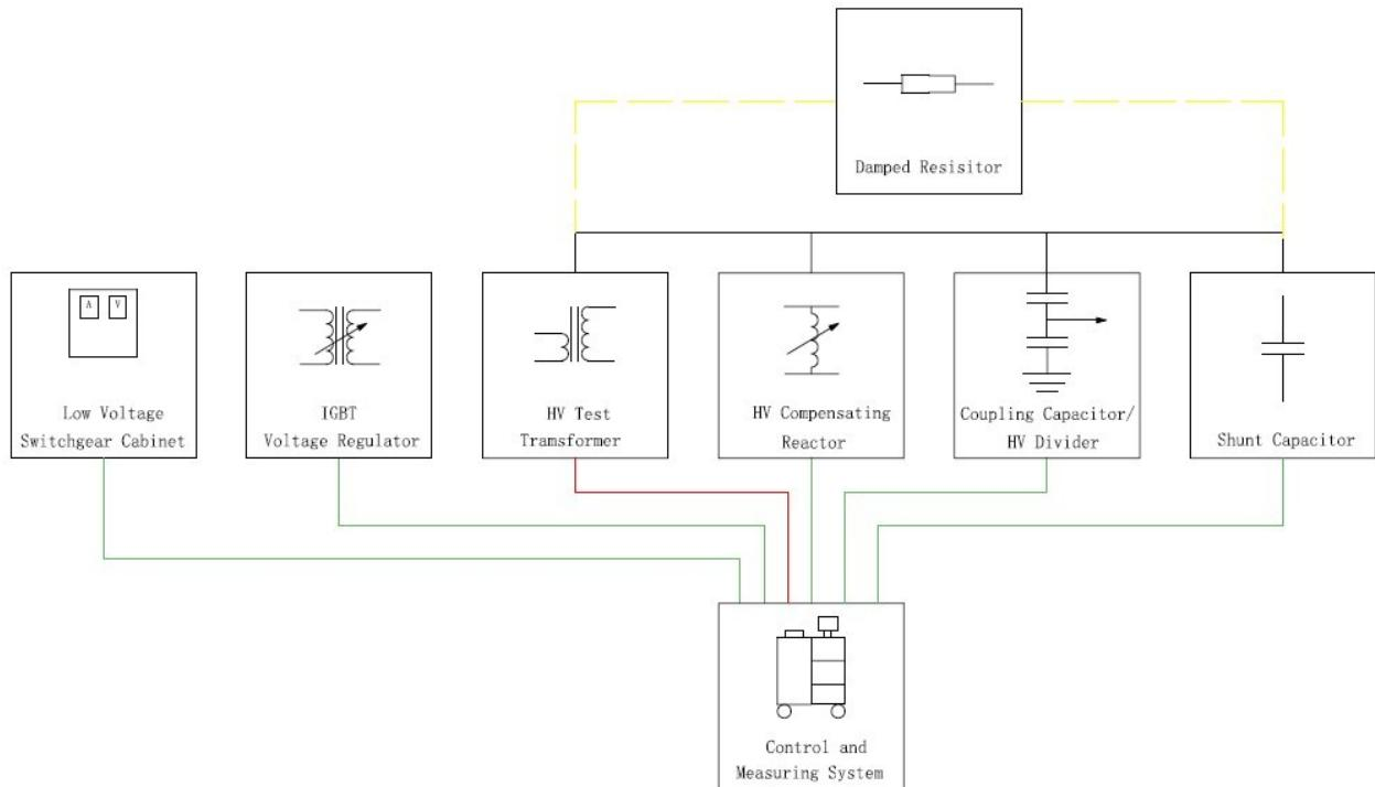
Compensating reactor use the viable inductance design, from minimum inductance to maximum inductance is has 20 times range, it is good for user to accuracy compensating to any shunt capacitor if the capacitance in the rated load. Also it can permit the test transformer in the lowest capacity rating. Instead of the traditional reactor, it can be viable inductance by motor, it need not any person to change any taps or bushing out by hand. It save time, also more safety.
