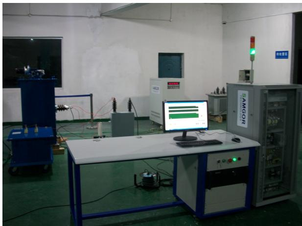
Over Voltage Cycle Test System is the type test, repeated over voltage from lowest rated voltage to the ambient temperature to improve the dielectric performance for the shunt capacitor above 10kV. In the recent year, this test is more popular to done in the modern factory.
